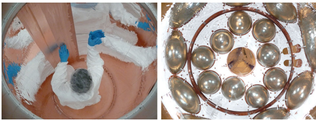
Fig. 2 Left cryostat being lined with VM2000 mirror foil. Right bottom view of the PMTs inside the cryostat
